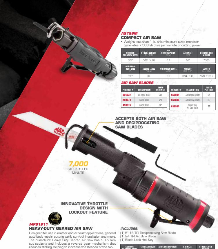
Features a lockout throttle design, 360° rotating exhaust that can direct air away from the user, and rubber grip that is resistant to most common automotive fluids. Another key feature of the Heavy Duty Geared Air Saw is it accepts both air saw and reciprocating saw blades, for added versatility.
